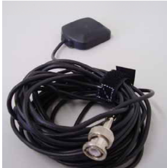
Figure 5: A GPS antenna with 15' cable
