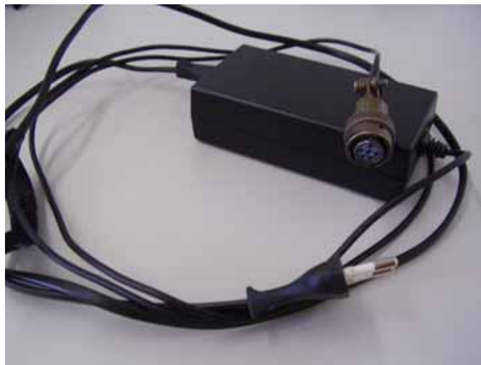
Figure 4: 12V power supply cable
