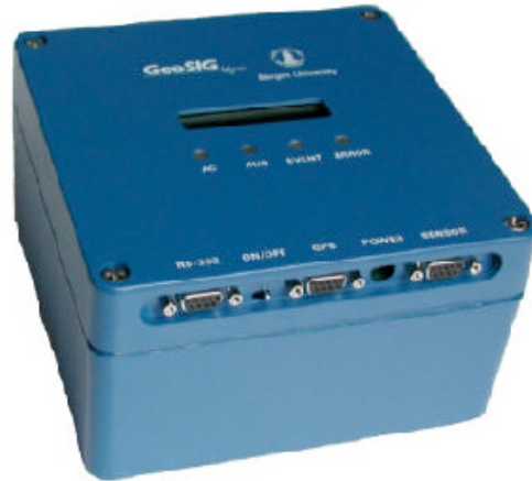
Figure 5.11 The GeoSig compact seismograph with 3 built in 4.5 Hz sensors. Note the standard computer connectors. In the middle on the lid is located a display giving alphanumerical info and 4 LED's give operational info. This is the most compact complete seismograph on the market.
