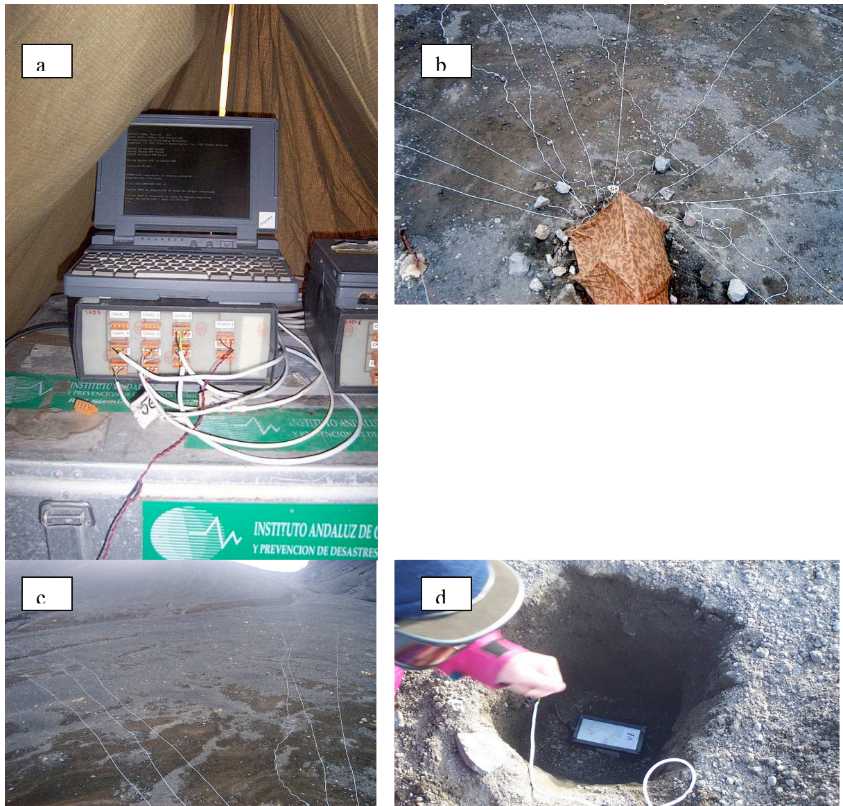
Figure 9.9 Some views of the portable array described above operating in the Antarctic Deception Island. a) The central unit is composed of a box with antialias filters, data acquisition card and GPS receiver and the laptop PC, which controls the conversion and save the data on disk. In this case two such subarray central units are installed in a tent for protection. b) An external view of the tent and the sensor cables. c) The cables are simply extended on the surface. In some cases it may be necessary to bury them for protection against the local fauna. d) One of the small sensors used is buried about 0.5m deep. The geophone is enclosed in a box containing the preamplifier-equalizer, which modifies its response to simulate a 1 Hz sensor.
