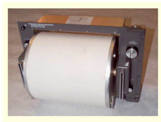
Figure 5.3 An example of a helicorder. The unit consists of a rotating drum with paper, a pen mounted on a pen motor that translates from right to left as the drum rotates. The gain of the pen amplifier is variable to adjust to different noise conditions. This recorder is made by Geotech (Model Helicorder RV-301B)
