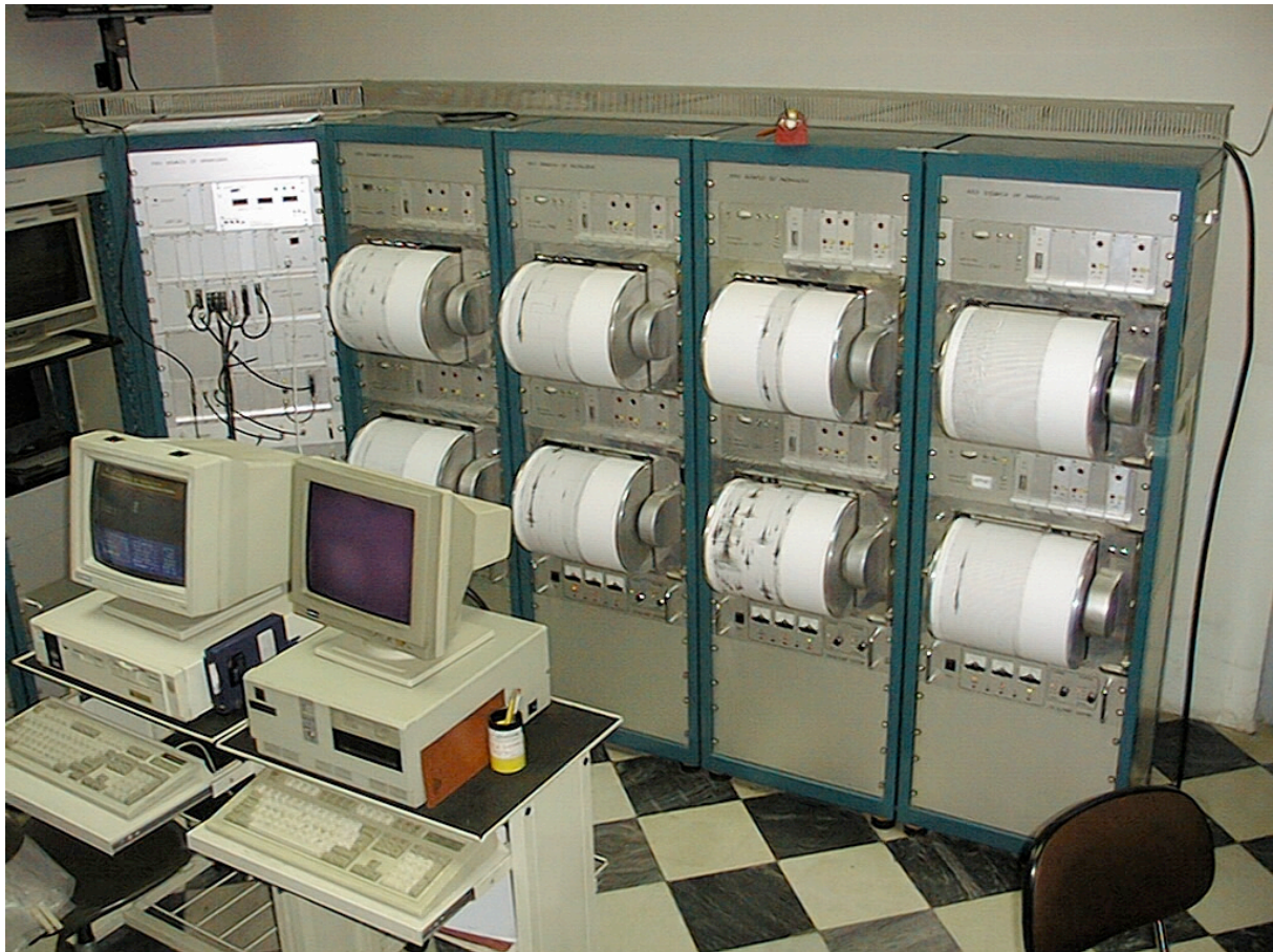
Figure 1.6 The central recording site at the Andalusia Seismic Network. The network consists of analog seismic station sending analog signals to the central recording site. Here the signals are digitized using the PC and events triggering the system are stored on disk. In addition, data are recorded in analog form on drum recorders (helicorder). In this photo we see an example where a seismic swarm is recorded making it possible to get an easy overview of the recent activity.
