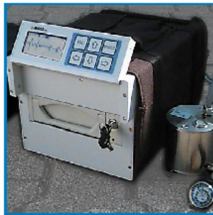
Figure 5.10. The Lennartz MARSliteHD recorder. Below the display is seen the 3.5" extractable hard disk. The model with magneto-optical recording is less than half the size (bottom part missing).
