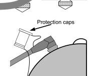
Mate both protection caps (cable and sensor) together. This prevents them from collecting dirt.
