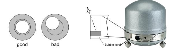
Finally tighten all three feet by turning their counter nuts clockwise until they lock firmly. Check it. A loose foot will strongly compromise the signal quality.
