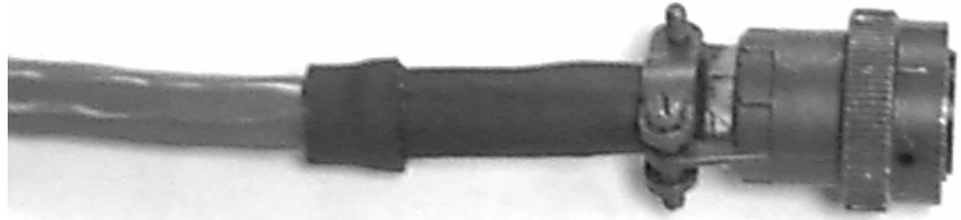
Figure 36: Completed assembly of recorder-end of cable 840356
