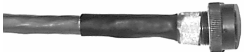
Figure 35: Shrink-n-Shield tubing in correct position (after shrinking)
