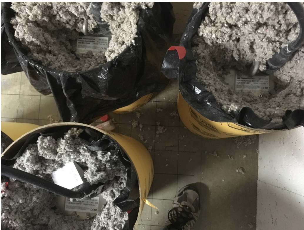
Figure 4 Picture of installed seismometers, overhead
